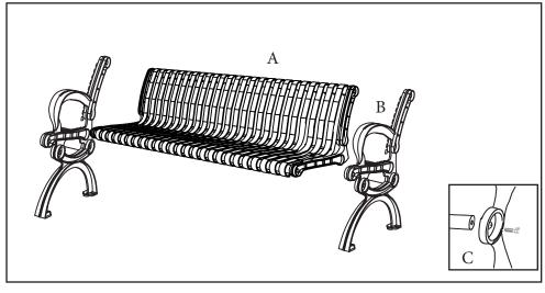
1. Assemble the seat supports(B) and the seat (A) with bolts and washers (C).
