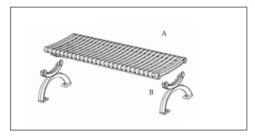
1. Assemble the seat supports(B) and the seat (A) with bolts and washers (C). Insert bolts (C) loosely.
