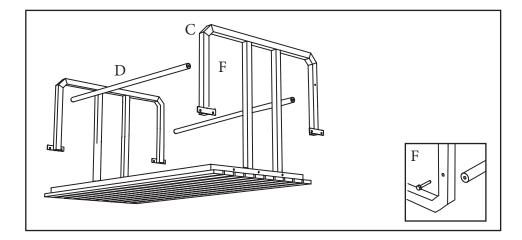
3. Connect table brace (D) to the middle of table support (C) with bolts (E) loosely.
