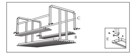
4. Connect seats with seat supports(C), and insert bolts (E) loosely.
